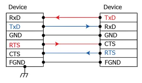
Note: FGND is the frame ground that is soldered to the metal shield on the DB-9 cable.
