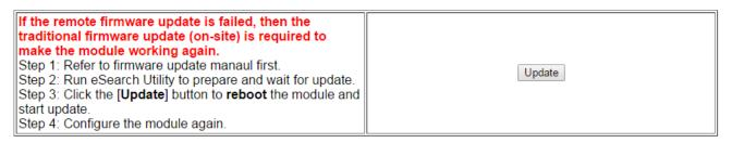
Firmware update requires initialization and local network operations. Traditional firmware update requires adjusting the Init/Run Switch and reboots the module manually for the initialization of firmware update, while new firmware allows user to initialize the module via web interface without adjusting the hardware switch. Initialization via web is useful when module is installed in remote site and can be accessed by a remote PC via TeamViewer.
