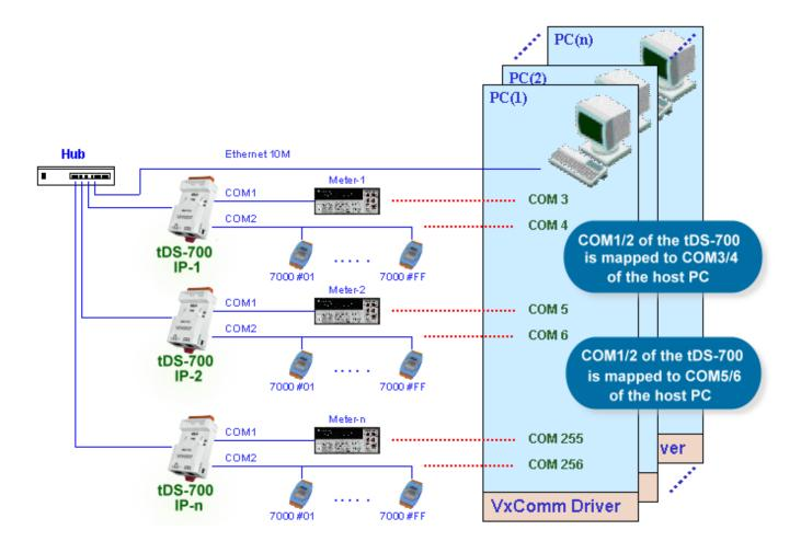
In the configuration above, Meter-1 is virtualized to link to COM3 of the host PC. Therefore, a program originally designed for the MS-COMM standard can access the meter without the need for any modification.
