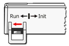
**Step 4** Reset the Init/Run switch on the tDS-700 module to the **"Run"** position and reboot the device.
