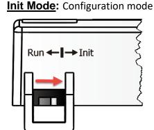
For tDS-700 series modules, the operating mode switch is set to the **Run** position by default. In order to update the firmware for the tDS-700 series module, the switch must be moved from the **Run** position to the **Init** position. The switch must be returned to the Run position after the update is complete.
