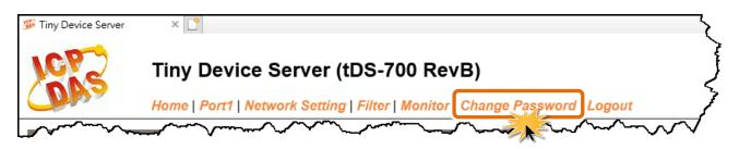
After clicking the **Password** tab, the **Change Password** page will be displayed. To change a password, first enter the old password in the **"Current password"** field (use the default password "admin") and then enter a new password in the **"New password"** field. Re-enter the new password in the **"Confirm new password"** field, and then click the **"Submit**" button to update the password.
