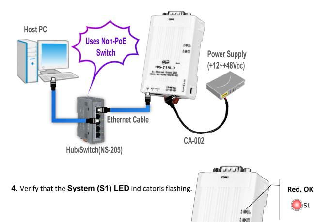
**5.** Perform a Self-test wiring check as follows:
